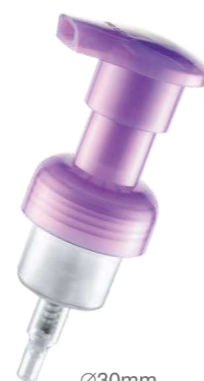
Ø30mm SM3105 Discharge rate: 0.40±0.06ml/T
