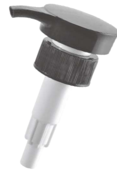
Ø33/410, Ø38/410 SM25A11 Discharge rate: 4.00±0.40ml/T
